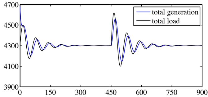
**Figure 4.3:** Evolution of the total power generation for the IEEE 118 bus example under the  $\text{dac}+\text{L}\partial$  dynamics for the communication digraph  $\mathcal{G}$ , design parameters  $\nu_1 = 1$ ,  $\nu_2 = 1.3$ ,  $\alpha = 10$ ,  $\beta = 40$  and  $\epsilon = 0.0086$ , and time-varying total load. The example depicts the input-to-state stability of the mismatch dynamics.
