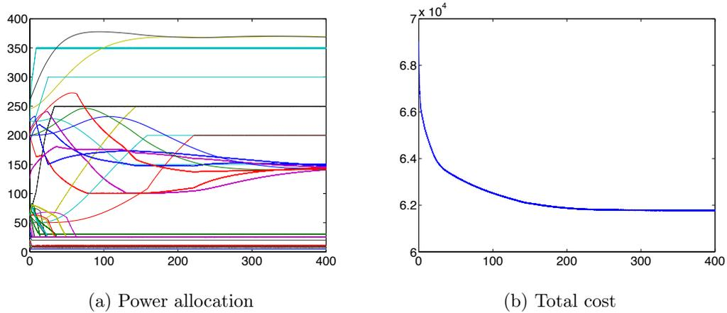
**Figure 3.1:** Evolution of the power allocation (a) and the network cost (b) under the Laplacian-nonsmooth-gradient dynamics in the IEEE 118 bus test case. The stepsize of the Euler time-discretization is  $2.5 \times 10^{-3}$  and  $\epsilon = 0.006$ .
