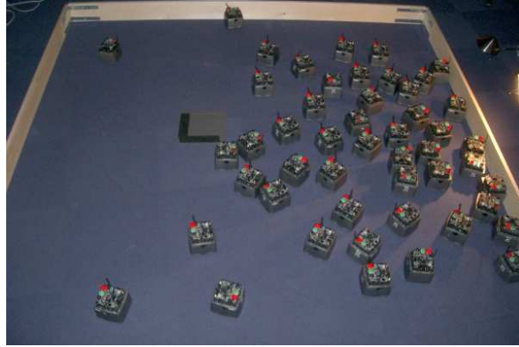
Figure 1.1: Robot swarm developed at MIT. Image courtesy [60], see also [61]
