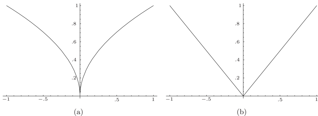
Figure S1. Illustration of the difference among continuous, locally Lipschitz, and differentiable functions. (a) shows the graph of f : \mathbb{R} \rightarrow \mathbb{R} , f(x) = \sqrt{|x|} , which is continuous at 0, but not locally Lipschitz at 0. (b) shows the graph of f : \mathbb{R} \rightarrow \mathbb{R} , f(x) = |x| , which is locally Lipschitz at 0, but not differentiable at 0.
