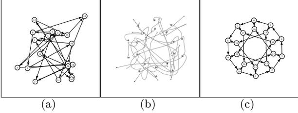
Fig. 4. Execution of the algorithm (18) with  $h = .25$  and  $\sigma = .2$  over a relative sensing network in  $\mathbb{R}^2$  composed of 20 agents. (a) initial configuration, (b) evolution, and (c) formation after 80 iterations.
