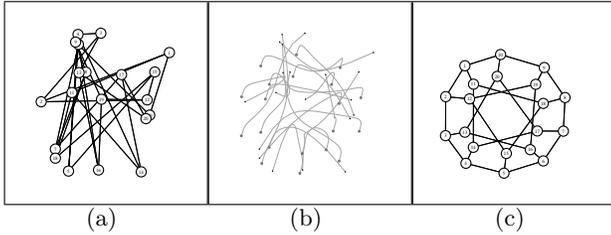
Fig. 5. Execution of the algorithm (10) with  $h = .25$  over a relative sensing network in  $\mathbb{R}^2$  composed of 20 agents under errors in the orientation of the agent frames. (a) initial configuration, (b) evolution, and (c) final formation shape.
