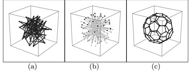
Fig. 2. Execution of the algorithm (10) with  $h = .25$  over a relative sensing network in  $\mathbb{R}^3$  composed of 60 agents. (a) initial configuration, (b) evolution, and (c) final formation.
