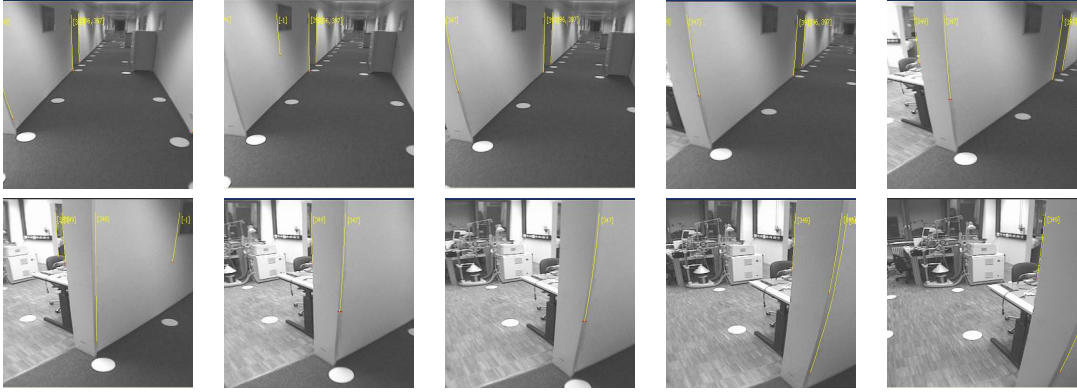
Figure 8: An example of the images used by the 9 robots during the navigation to test the proposed method [35]. Although the data set also provides artificial landmarks (white circles on the floor), we test the algorithm using the lines extracted from natural landmarks (in yellow).
