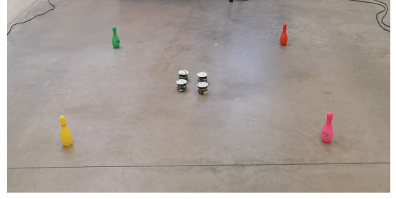
Fig. 5. Experimental setup: 4 ePucks and their corresponding targets.
