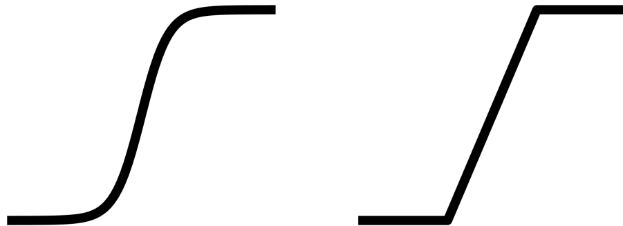
Figure 3. The sigmoidal (left) and linear-threshold (right) activation functions are commonly used for defining firing rate models.
