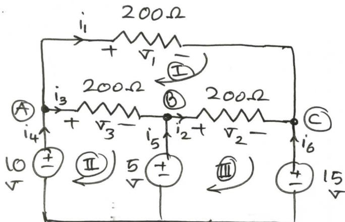
b) Loop I:  $V_1 - V_2 - V_3 = 0$
