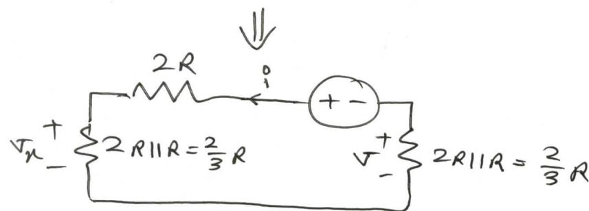
Voltage division:  $V_{L2} = \frac{2/3 R}{2R + 2/3 R + 2/3 R} \times V_S = 0.2 V_S$
