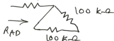
$$\Rightarrow R_{AD} = (100 \parallel 100) + 33 = 83 \text{ k}\Omega$$
