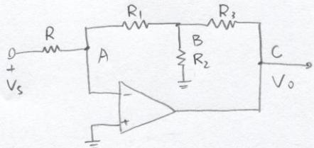
a) This is neither an inverting nor a non-inverting OpAmp. We need to use node voltage analysis to solve the problem
