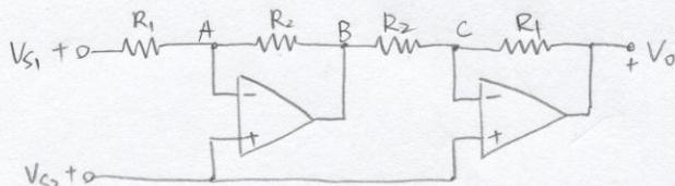
From equations of an ideal OpAmp:  $V_P = V_N \Rightarrow V_A = V_{S1}, V_C = V_{S2}$
