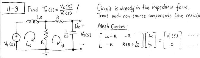
Circuit is already in the impedance form. Treat each non-source components like resistors.
