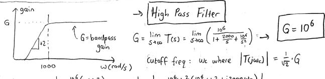
$$\begin{aligned} \left| T(j\omega_c) \right| &= \left| \frac{10^6 (-\omega_c^2)}{-\omega_c^2 + j 2000 \omega_c + 10^6} \right| = \left| \frac{-10^6 \omega_c^2 (10^6 - \omega_c^2 + j 2000 \omega_c)}{(10^6 - \omega_c^2)^2 + (2000 \omega_c)^2} \right| \\ &= \frac{10^6 \omega_c^2}{((10^6 - \omega_c^2)^2 + (2000 \omega_c)^2)} \left( (10^6 - \omega_c^2)^2 + (2000 \omega_c)^2 \right)^{1/2} = \frac{40^6}{\sqrt{2}} \end{aligned}$$
