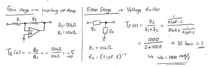
However, when plugged into the circuit, the source internal resistance and the load resistance will affect the transfer functions in a bad way.
