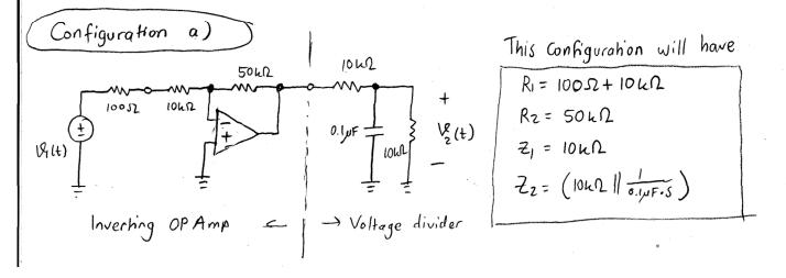
$$T_{G_Q}(s) = -\frac{R_2}{R_1} = \frac{-50 \, \text{k} \Omega}{10.1 \, \text{k} \Omega} = -4.95$$
