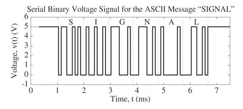
Bits are sent sequentially, they are preceded by a *start* bit followed by one or two *stop* bits
