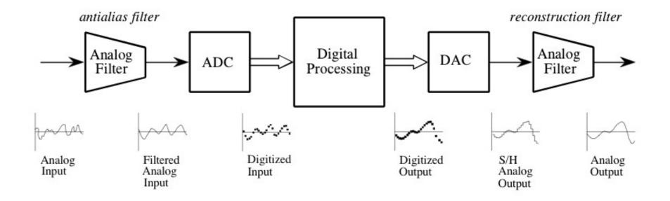
Analog electronic filters are used to comply with the sampling theorem. The filter placed before ADC is an antialias filter. It removes frequencies higher than half the sampling rate. The filter placed after the DAC is a reconstruction filter. It may include a correction for the zeroth-order hold.
