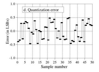
**The quantization error looks very much like random noise.** Because of this, it is usually modeled as a random number between – ½ and ½, with zero mean and standard deviation of 1/sqrt(12) LSB (uniform probability distribution)
