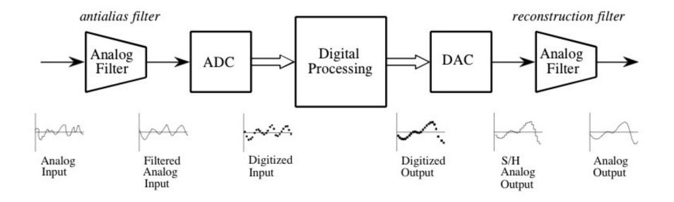
Analog filters are not ideal! Thus, knowledge of lowpass filters is important to be able to deal with different types of signals (analog filters are being substituted by digital ones)
