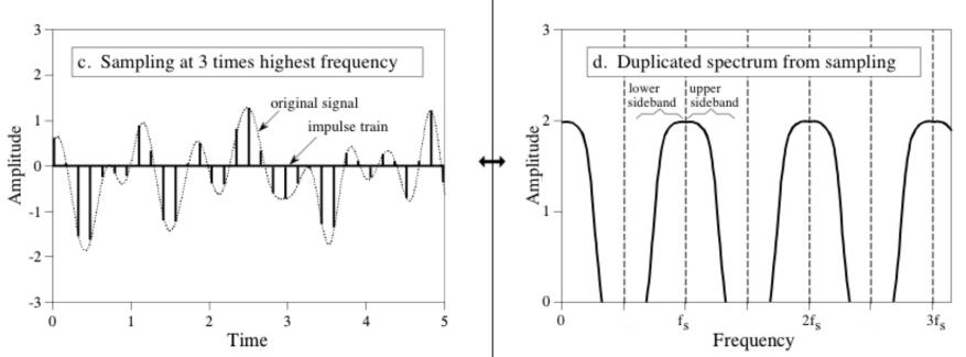
As you can see, the sampling has the effect of **duplicating the spectrum** of the original signal an infinite number of times. In other words, **sampling introduces new frequencies**
