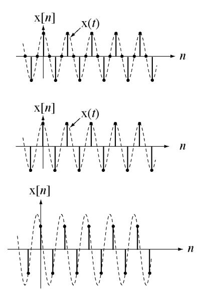
Cosine sampled at twice its Nyquist rate. Samples uniquely determine the signal.
