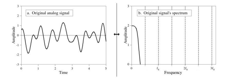
Here the analog signal has a frequency of  $0.33 \times f_s < 0.5 \times f_s$
