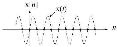
Adding a sine at the Nyquist frequency (half the Nyquist rate) to any signal does not change the samples. Sine sampled at its Nyquist rate. All the samples are zero.
