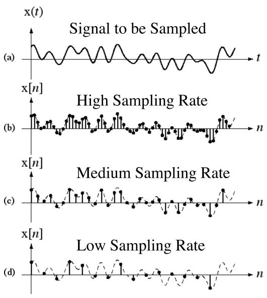
Suppose you sample a signal in some way. If you can **exactly reconstruct** the signal from the samples, then you have done a **proper sampling** and **captured the key** signal **information**
