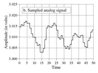
Before:  $t \in \{0, 0.1, \dots 50\},$  $y_A(t) \in (3000, 3025),$  After quantization:  $t \in \{0, 0.1, ..., 50\}$ ,  $y_Q(t) \in \{3000, 3001, ..., 3025\}$
