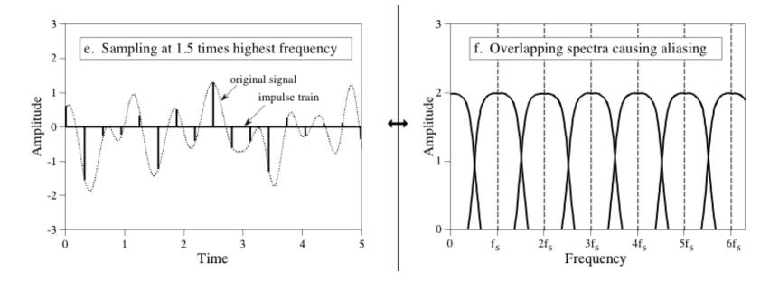
Here,  $f = 0.66 \times f_s > 0.5 \times f_s$ , so this is an improper sampling. In the FD this means that the repeated spectra overlap. Since there is no way to separate the overlap, the signal information is lost
