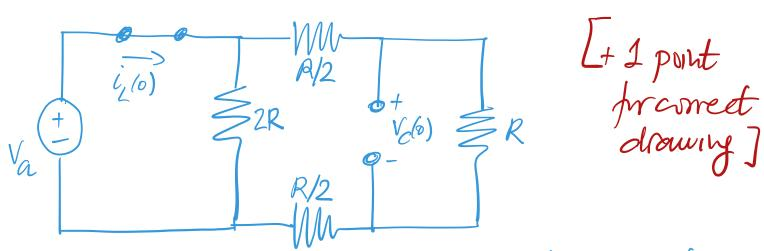
To find out i/10), we combine the three resistors in series. The resulting resistor is in parallel with 2R.
