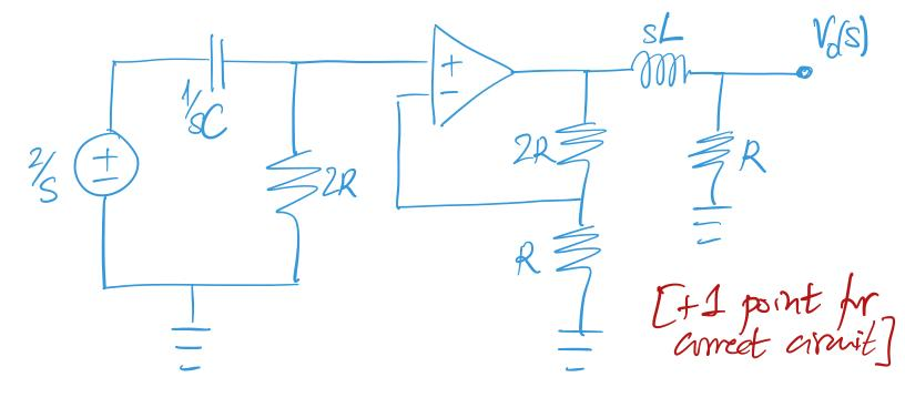
The trunsfer function can be found by realizing this is the composition of a voltage divider, a non-inverting op-amp, and another voltage divider. The presence of the normal methy op-amp ensures there is no body.
