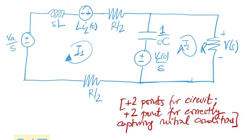
We use mesh correct analysis, as method. We write equations by inspection
