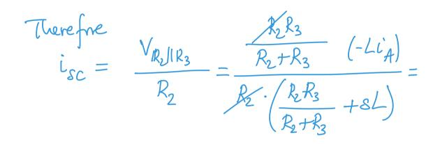
$$= \frac{-R_3 Li_A}{R_2 R_3 + sL(R_2 + R_3)}$$
