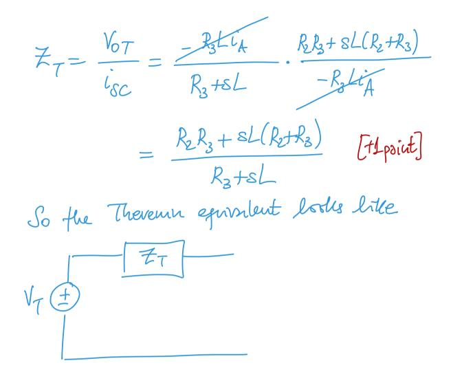
2.- Part I We convert the circuit to the s-domain, using a current source to take care of the initial condition (since we are going to vse nodal analysis).
