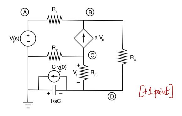
Now, we only have 1 voltage source to table care of. With the choice of groond, we actually have  $V_A = V_i(s)$  [71 point] Therefore, we only need to write KCL for modes B, C, and D.
