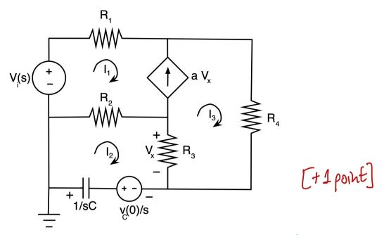
We have one problem to take care of, the arrent source. Since it belogs to two meshes, we use a supermesh, defined sy  $I_1 - I_3 = -aV_X$  [+1 point] KVL for the supermesh is  $R_1 \cdot I_1 + R_4 I_3 + R_3(I_3 - I_2) + R_2(I_1 - I_2) = V_1(s)$ We also write KVL for mesh 2  $R_2(I_2 - I_1) + R_3(I_2 - I_3) - \frac{V_c(0)}{S} + \frac{1}{8C} \frac{I_2}{E+1} = 0$ Finally, we deal with the presence of the
