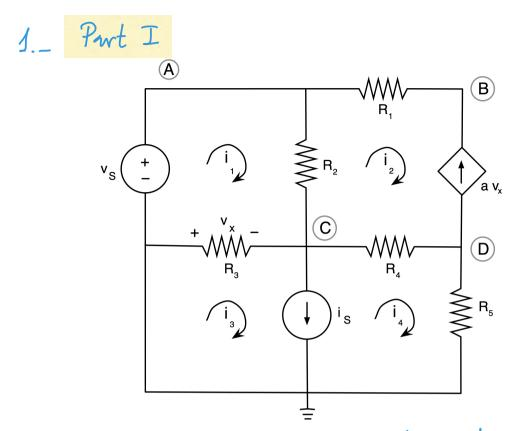
Looking at the circuit, we observe the presence of 2 correct sources, which are problems we need to deal with to use mesh correct analysis. One of them only belongs to one much (method 2), but the other selongs to two, so we will use a supermuch for it (method 3). So, method 2 for the current source on the right yields  $i_2 = -aV_X$  [+1 point] The supermech epintron is  $i_3 - i_4 = i_S$  [+1 point]
