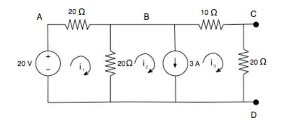
Set up mesh analysis equations
