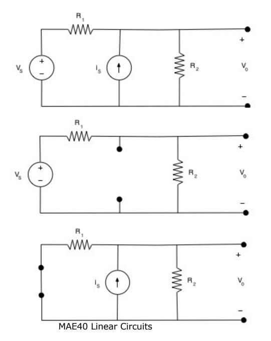
Find  $V_0$  using superposition  $V_0 = \frac{R_2}{R_1 + R_2} V_s + \frac{R_1 R_2}{R_1 + R_2} i_s$
