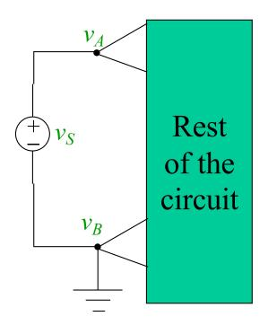
This removes the  $v_B$  variable (plus we know  $v_{A=}v_S$ ) – simpler analysis But can be done once per circuit
