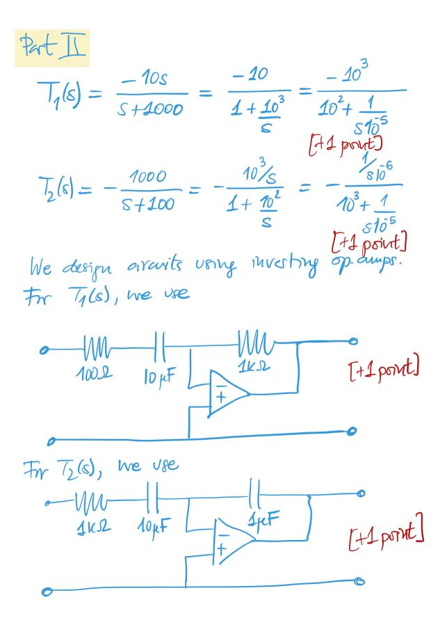
Part II Since T(s) is the som of T<sub>1</sub>(s) and T<sub>2</sub>(s), we consome the <u>two availe</u> in Part II in purallel to design (F1 point)
