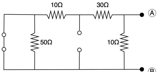
where the current source gets replaced Sy an open avail and the voltage source by a dond circuit. Next, we use association of resistors to find the equivalent resistance. Note that the SOL resistor is in parallel with a OLL resistor, so we can instead draw
