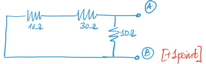
We consure the two resistors in series to get the plot
