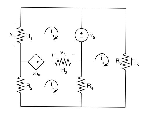
Looking at the circuit, we observe the presence of 1 correct source, which is a problem we need to deal with to use mesh arrent analysis.
